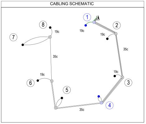
IF SUFFICIENT CABLE SLACK THEN REUSE EXISTING CABLES IF NOT POSSIBLE THEN RENEW CABLES
