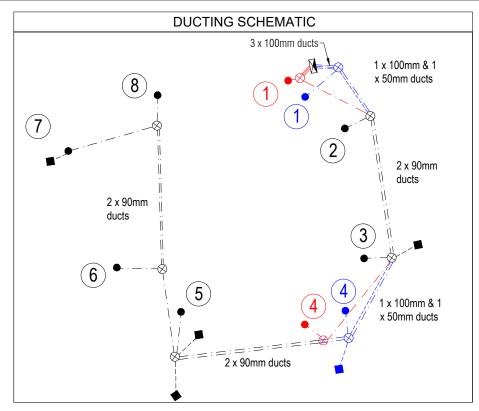
SIZE AND CONDITION OF DUCTS TO BE CONFIRMED ON SITE
